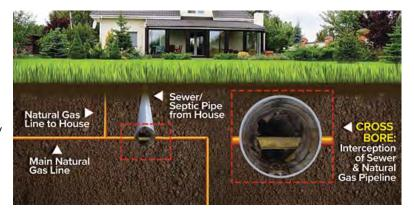
While cross bore incidents can impact any underground utilities, one of the most serious involves an intersection between sewer lines and natural gas lines. A cross bore is unintentional and can exist for years before a sewer line clogs or collapses.
